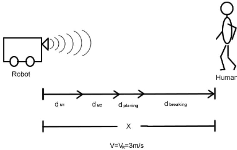
Fig 33: model of collision course scenario
