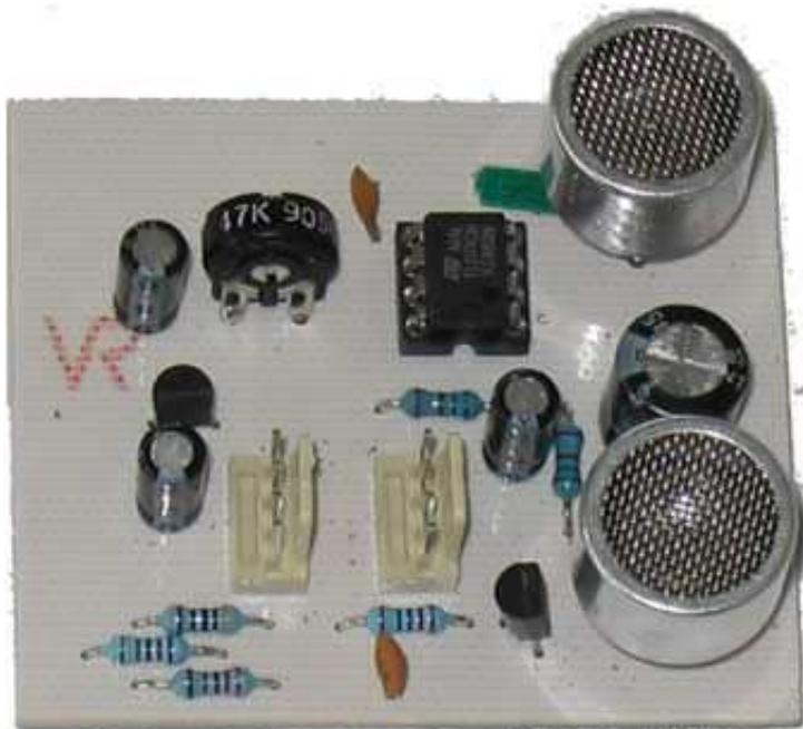
Fig 20: Ultrasonic sensor electronics (final design)
