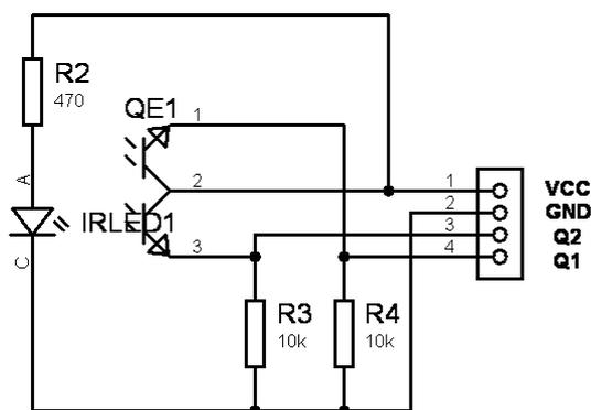
Fig 21: Shaft encoder circuit
