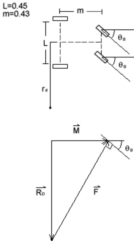
Fig 30: Steering kinematics
