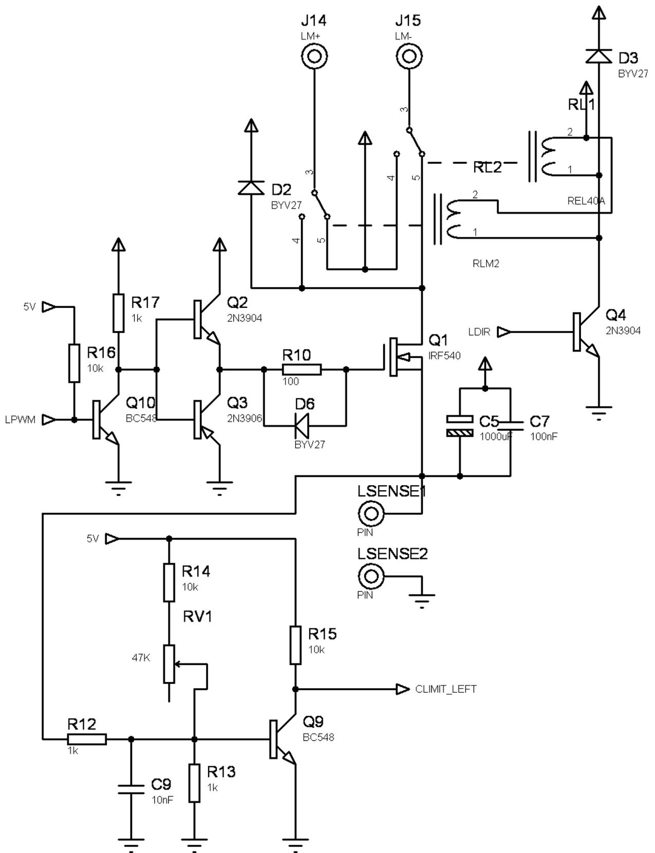
Fig 25: Left channel of the drive system electronics.
