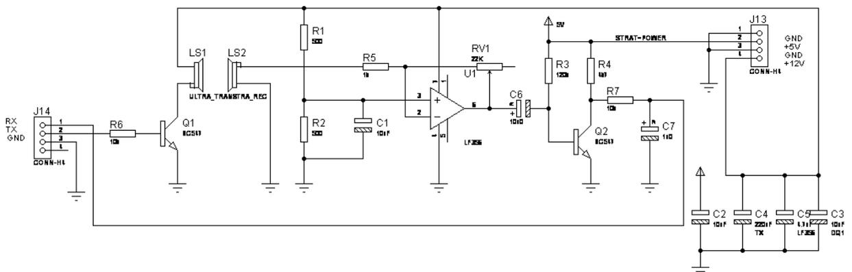
Fig 17: Ultra sonic distance measurement electronics
