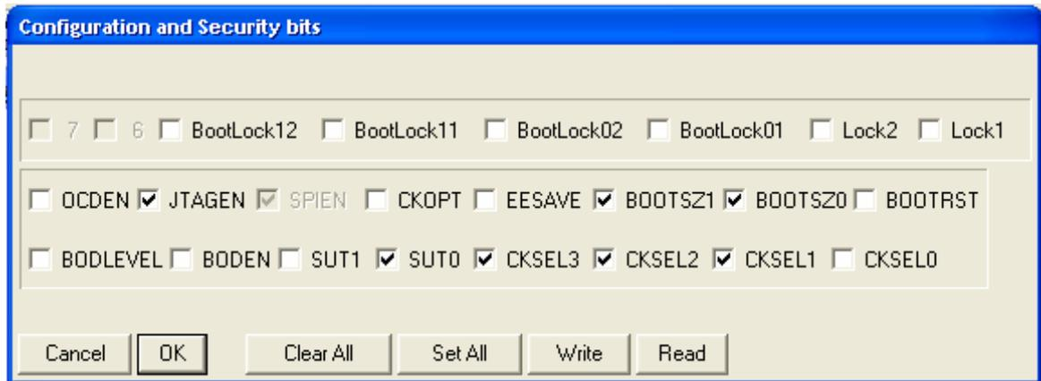
Fig 2.2 PonyProg Configuration bits
