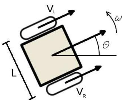
Fig 12: Differential driven Robot
