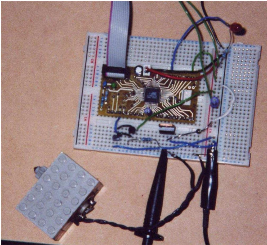
Fig 16: Atmel Mega16 Microcontroller board used for designing the motor controllers
