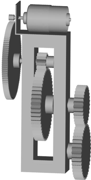
The two gearboxes are constructed out of 4 solid aluminium bars each, which are bolted together. On the bottom bar two slots are milled out, increasing the accuracy of their alignment with the other bars. During construction the bars were clamped together, in order to align the shaft holes of both bars precisely. The surfaces of the bars have been milled straight at the beginning, to have accurate reference during construction.
