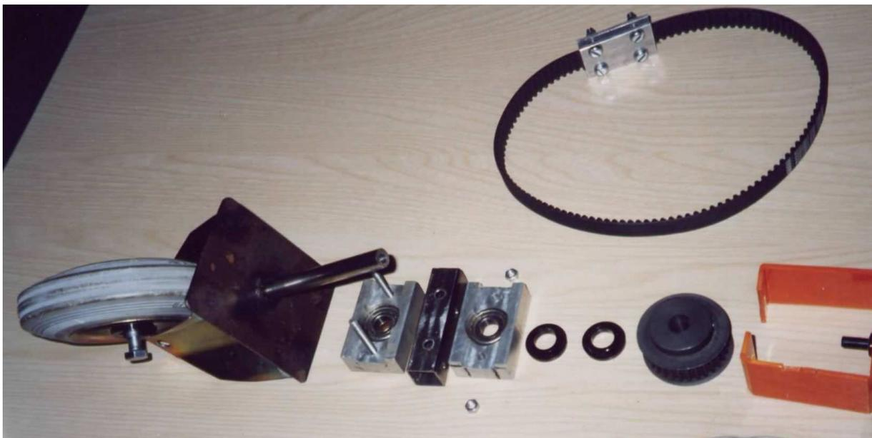
Fig 13: Explosion picture of one steering link
