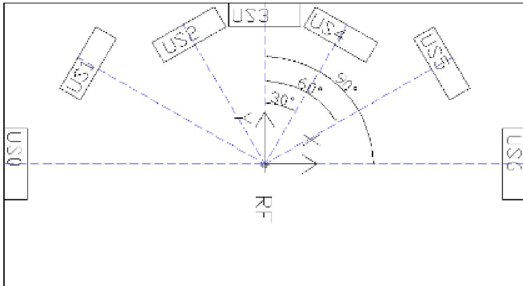
Fig 31: Position of the ultra sound transducers
