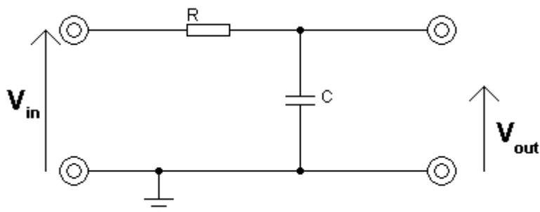
Fig 19: low pass filter (used in ultra sonic circuit)
