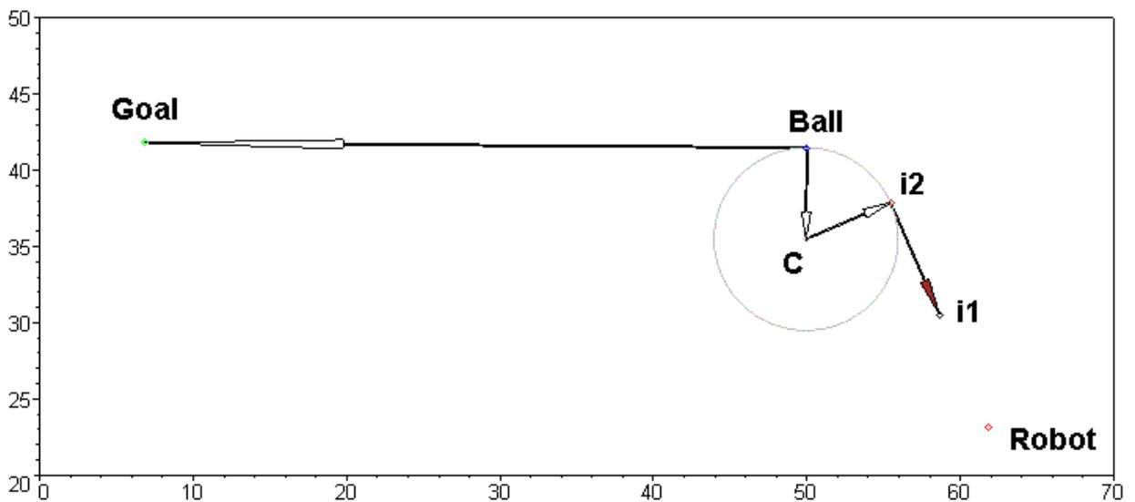
Fig 3: Circle and straight line move trajectory applied to robot football
