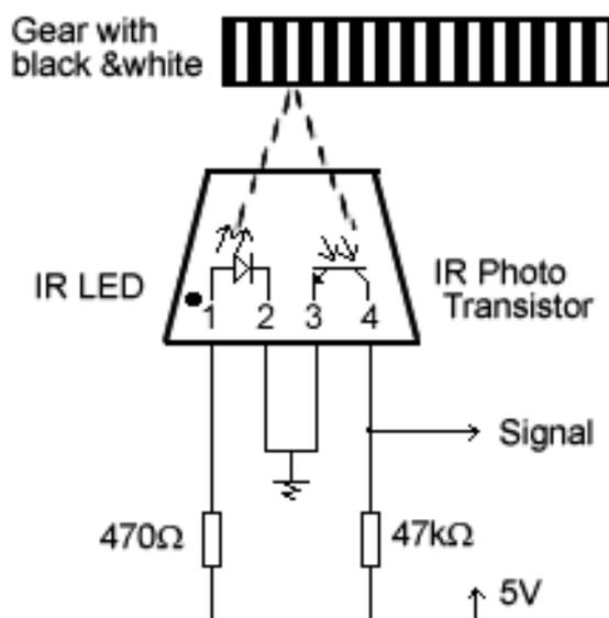
Fig 23: ISTS708 opto switch with circuit
