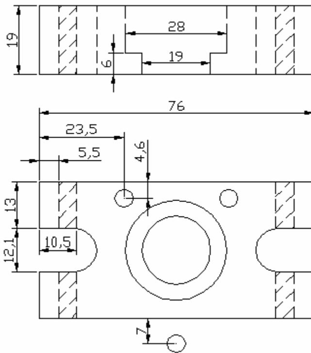
Fig 15: Housing with 3 holes for gearbox-mount
