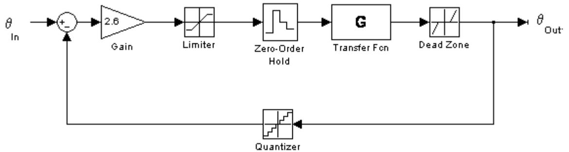
Fig 24: Steering controller model
